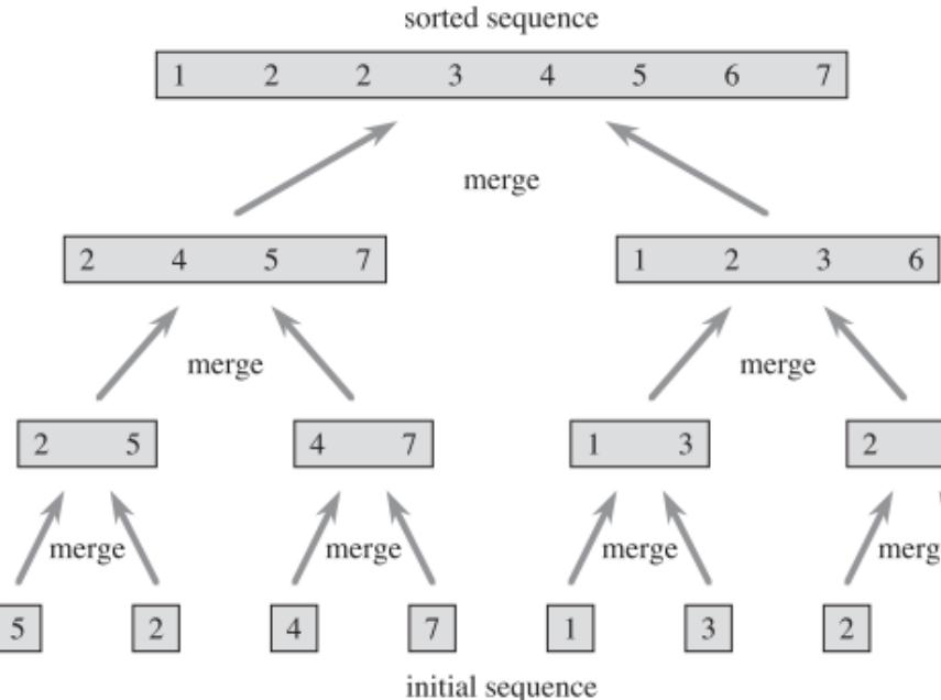
The operation of merge sort on the array A [5; 2; 4; 7; 1; 3; 2; 6], The lengths of the sorted sequences being merged increase as the algorithm progresses from bottom to top.
